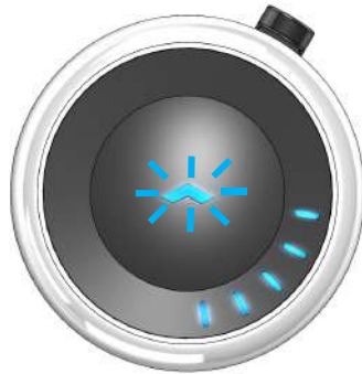
Figure 23. WHILL LED logo flashes when seat is forward
