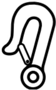
Figure 30. Tie down point marking
