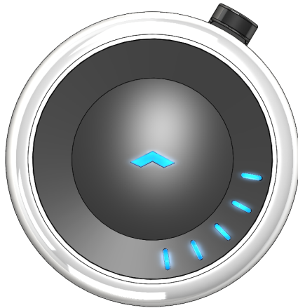
Figure 13. Lights indicating full battery charge.
