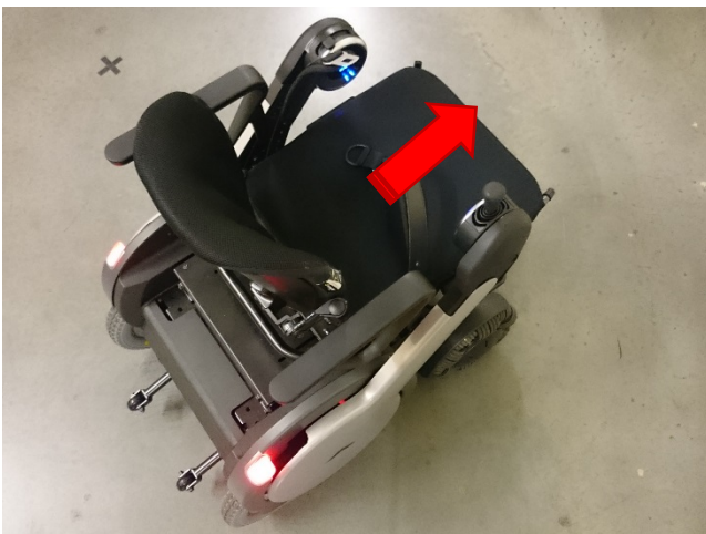
Figure 5. With the mode switch in the “S” position, slide the seat forward using directional controller. Turn the chair off.
