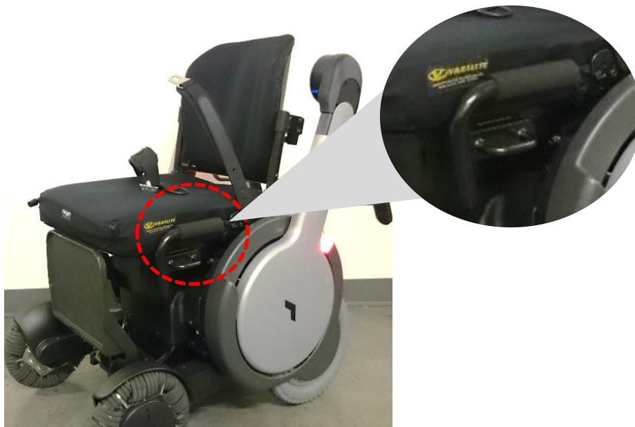
Figure 11. Pressure relief handle locations.
