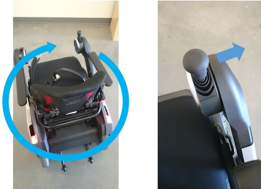
Figure 19. To rotate to the right (left figure) move the directional controller directly to the right (right figure).
