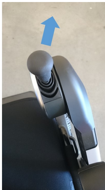
Figure 18. To turn to the right (left figure) move the directional controller at a diagonal (right figure).
