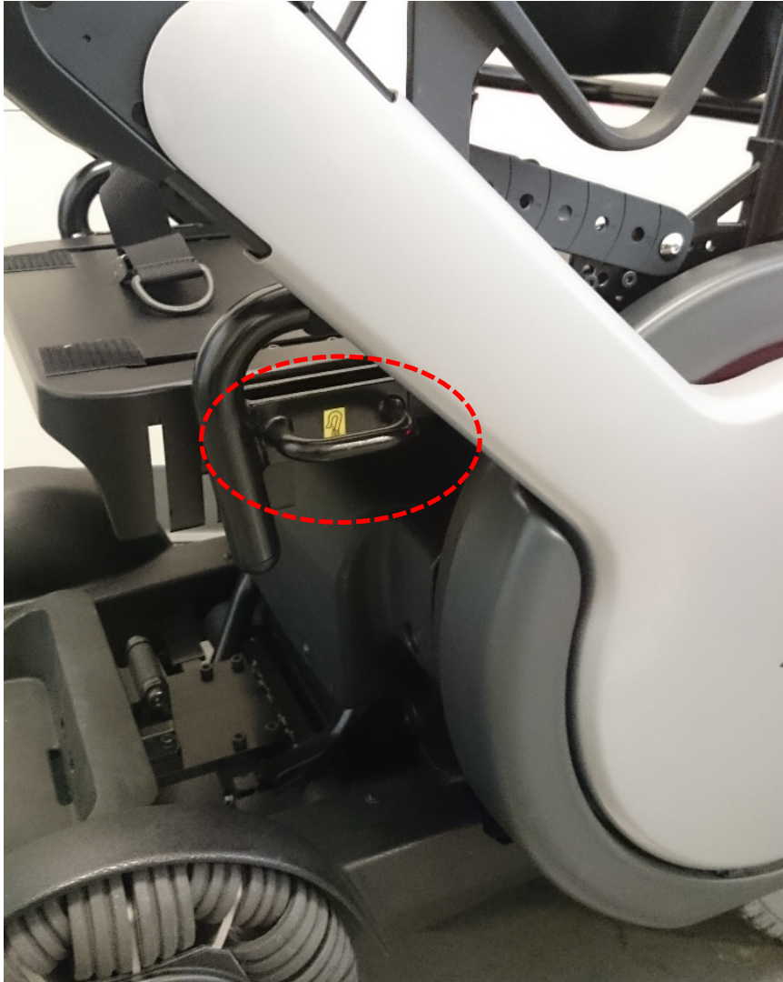
Figure 29. Front tie down point
