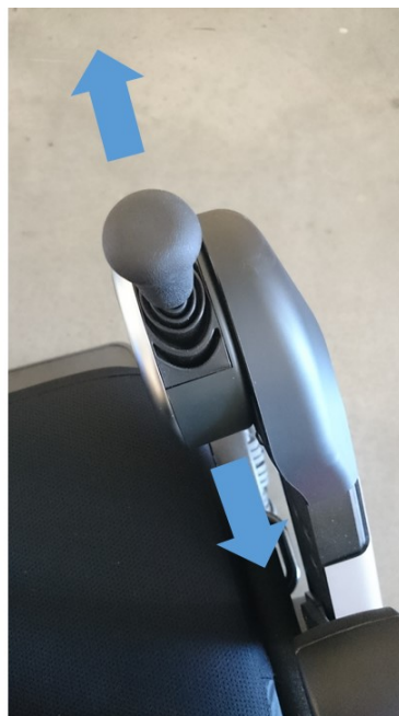
Figure 17. To drive the chair straight forward or backwards (left figure) move the directional controller forward or back (right figure).
