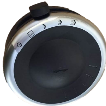
Figure 20. Mode switch placement for slow speed setting
