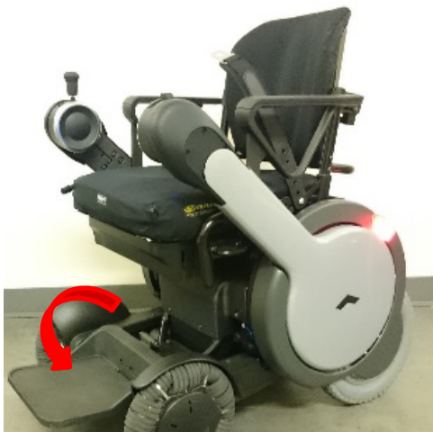
Figure 9. If footplate was pivoted up, return it to the horizontal position.
