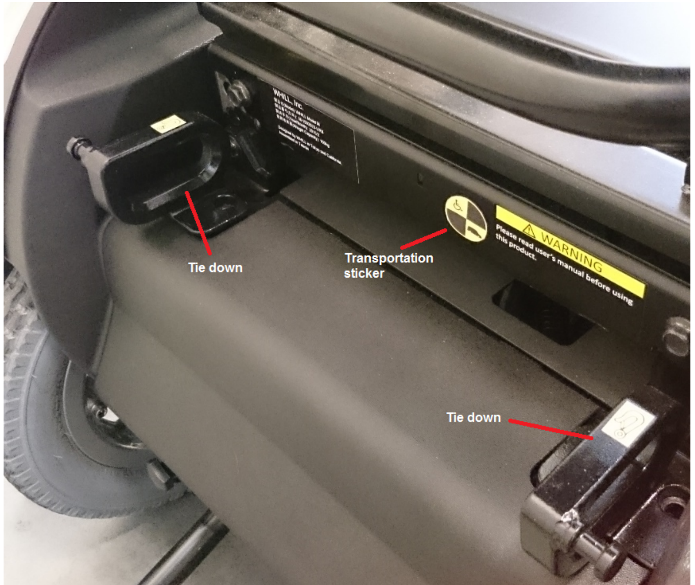
Figure 28. Rear view of wheelchair showing transportation sticker and tie downs
