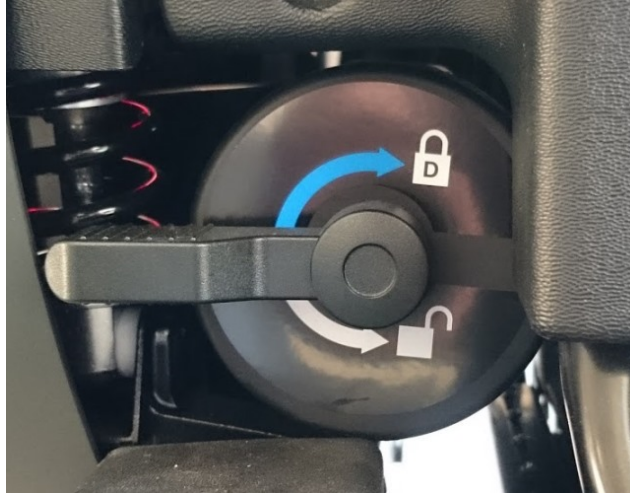
Figure 24. Close up of brake release lever
