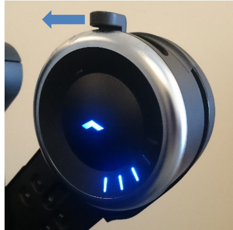
Figure 4. Be sure the chair is on. If needed, turn on the chair by pulling the mode switch all the way towards you
