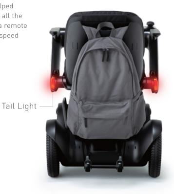
The tail light is clearly visible even with a bag hung over the back support, keeping you safe on the road at night.
